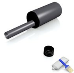
Insert internal drain connector into larger pipe, apply lubricant and push in smaller pipe.
