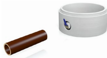
Apply lubricant to BKL joint.
