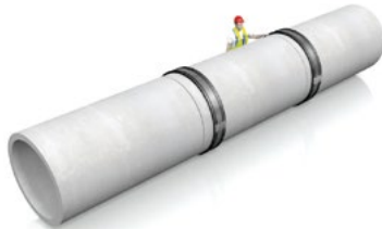
Slide coupling over one plain end.
