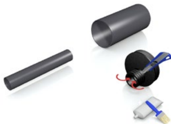
Fold in or cut off internal drain connector at the desired position, depending on the connection situation.
